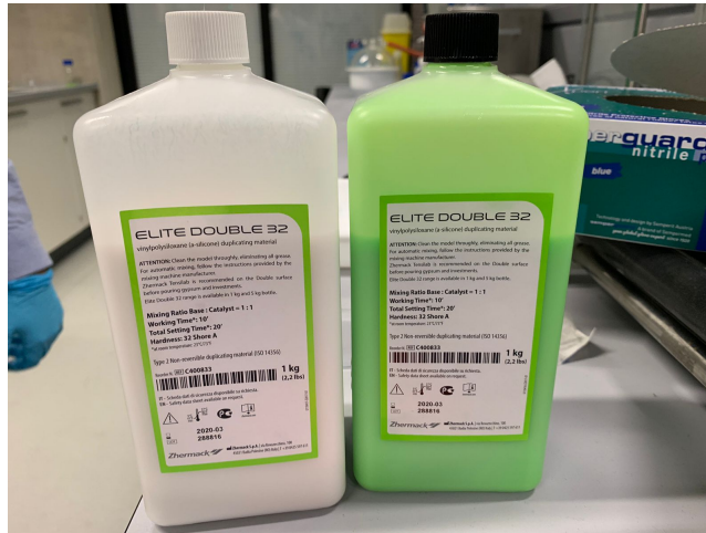
Figure 1: Base and Catalyst Containers of Elite Double 32. This material is used to cast the samples for the tensile tests to be performed.
