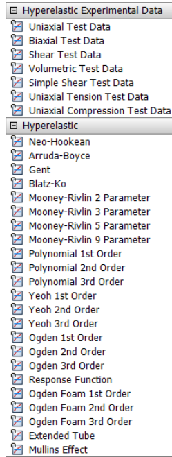
Figure 4: Hyperelasticity Models Available in ANSYS. Tabular experimental data or hyperelasticity coefficients can be used to define hyperelastic materials in ANSYS.
